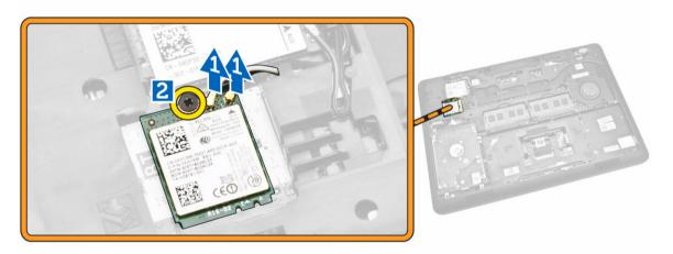
**4.** Remove the WLAN card from the computer.
