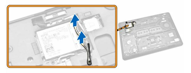
**4.** Remove the screw that secures the WWAN card [1] and remove the WWAN card from the computer [2].
