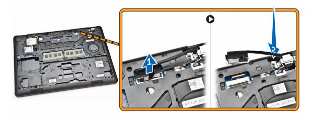
**6.** Remove the screws that secure the display assembly [1] and lift the display assembly to remove it from the computer [2].
