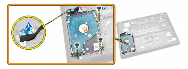
**4.** Remove the hard-drive assembly from the computer.
